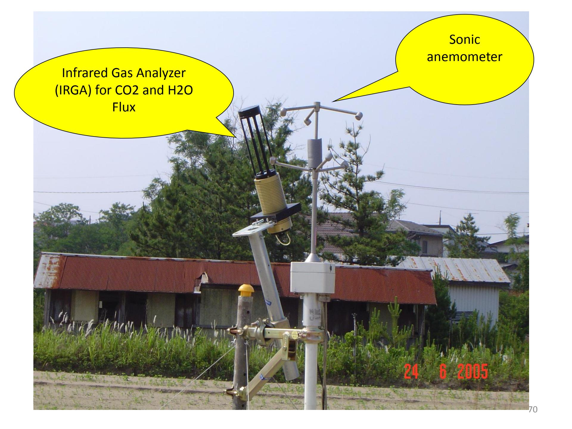
Infrared Gas Analyzer
