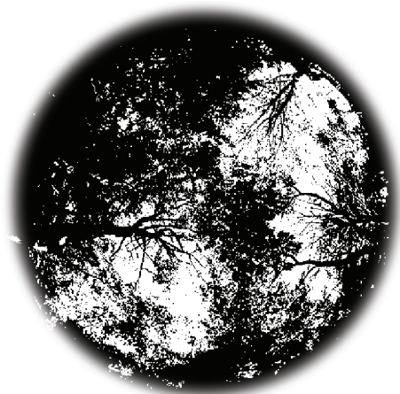
Figure 1.7b Digitalization of the fish eye photograph to determine the partition of visible sky on the photograph. 44 % of the sky is visible.
