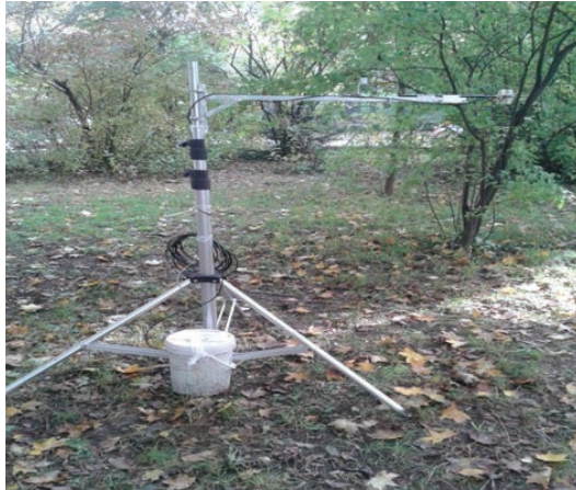
Figure 1.11 Instrumentation for measuring shortwave and longwave radiation balance in a canopy. A four component radiometer measures separately with 4 different optical sensors downward shortwave and longwave and upward shortwave and longwave radiation data are automatically stored using a datalogger which is installed in the bucket.
